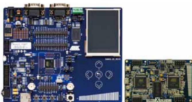
図2: SAM4S評価用ボード (左: SAM4S-EK、右: SAM4S Xplained Evaluation Kit)
